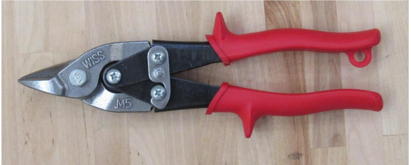
**About:** Snips are hand tools used to cut sheet metal and other tough webs. Compound-action snips use a compound leverage handle system to increase the mechanical advantage.
