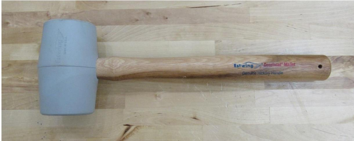
**About:** The rubber Mallet is used in woodworking or when a softer impact is required. The rubber head ensures that the face of the surface you are striking will not be damaged.
