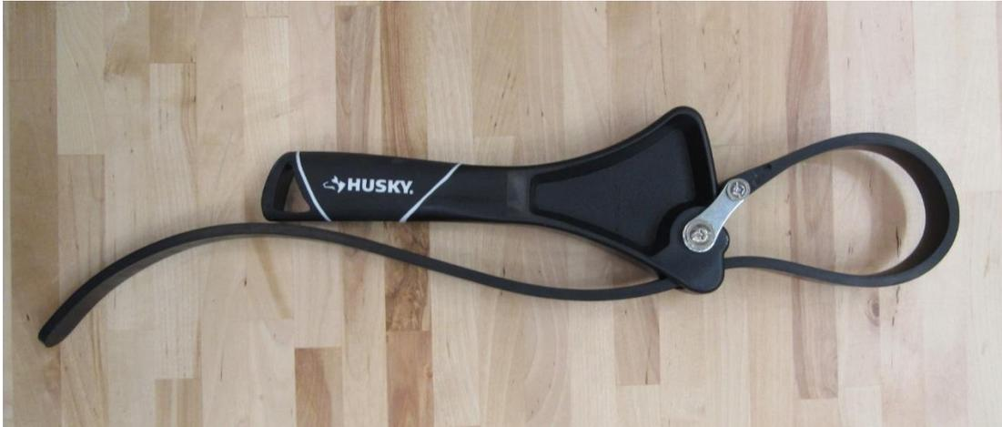
**About:** A strap wrench is any of various types of wrench that grip an object via a strap or chain being pulled in tension around it until it firmly grips. High static friction keeps it from slipping.
