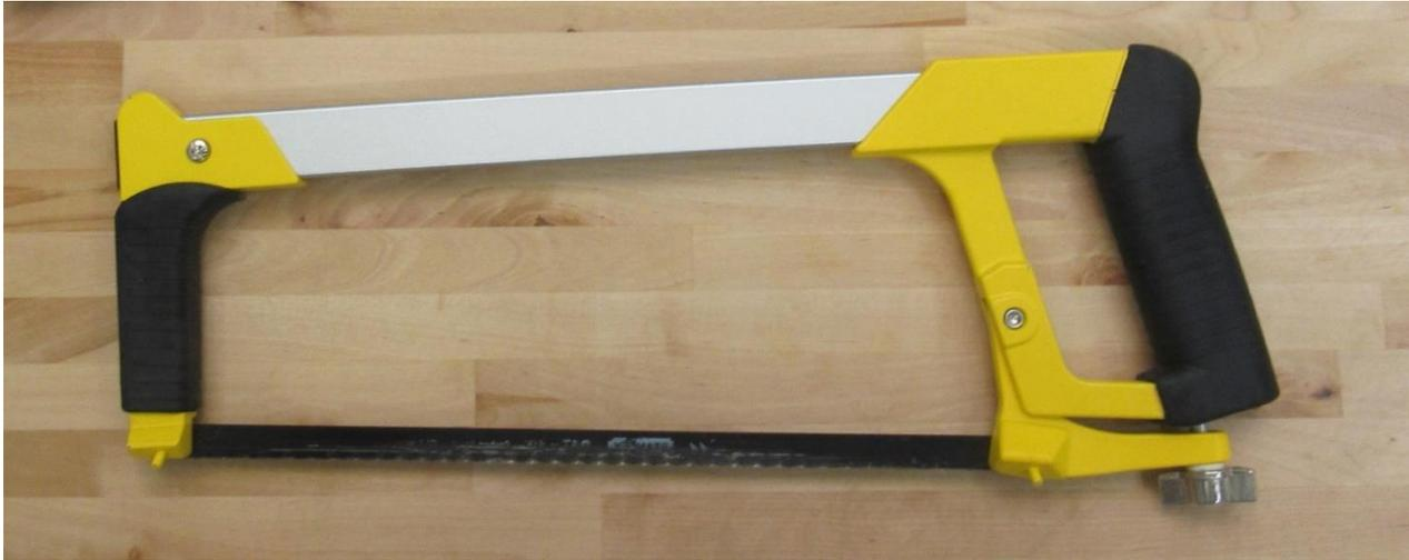
**About:** a fine-toothed tempered blade under tension, for cutting metal, bone, and other hard materials
