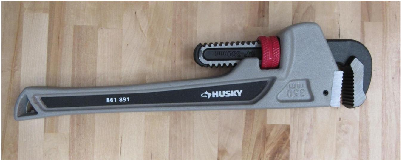
**About:** A plumber wrench is a pipe wrench used to rotate pipes used in plumbing. The wrench can easily be adjusted to different pipe diameters by rotating the key ring. This tool can close with significant force (without caution it is possible to dent or break the pipe) and thus does not need to engage a nut.
