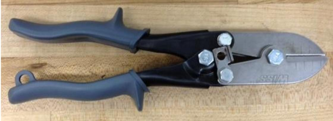
**About:** Quickly crimps round duct work for fittings
